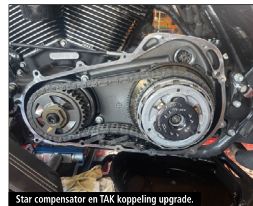
Star compensator en TAK koppeling upgrade.
